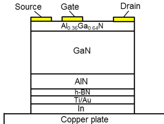
Figure 4. Schematic illustration of the transferred HEMT.
