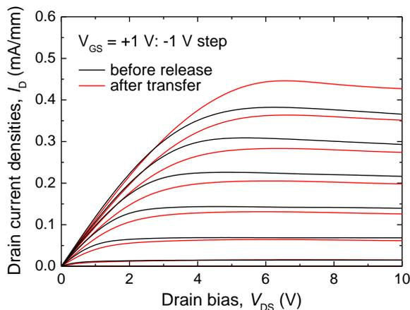
Figure 5.  $I_D$ - $V_{DS}$  characteristics of the HEMT before release (black solid lines) and after transfer to the copper plate (red solid lines).
