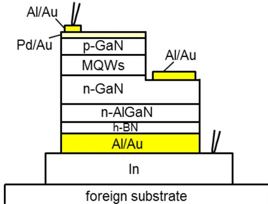
Figure 1. Schematic illustration of the transferred LED.
