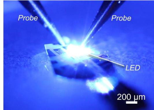
Figure 2. Photograph of blue-light electro-luminescence from the transferred vertical-type LED.
