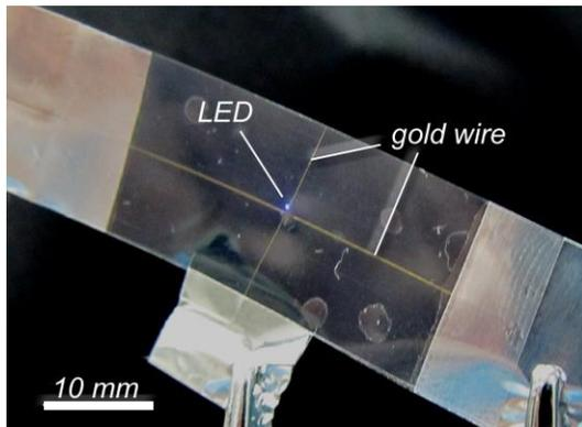
Figure 3. Photograph of the thin (< 0.1 mm) LED sandwiched by the commercially available adhesive tape.
