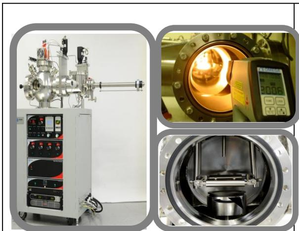
Fig. 1 Blue Wave HFCVD System with filament arrangement capable of reaching more than 2200°C for growth of diamond films.
