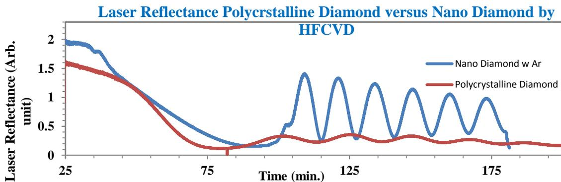
Fig. 5 Laser Reflectance graph showing comparison of nano and polycrystalline diamond after nucleation
