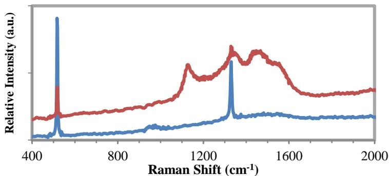
Fig. 4 Raman spectrum of nanodiamond, red, and polycrystalline diamond, blue.
