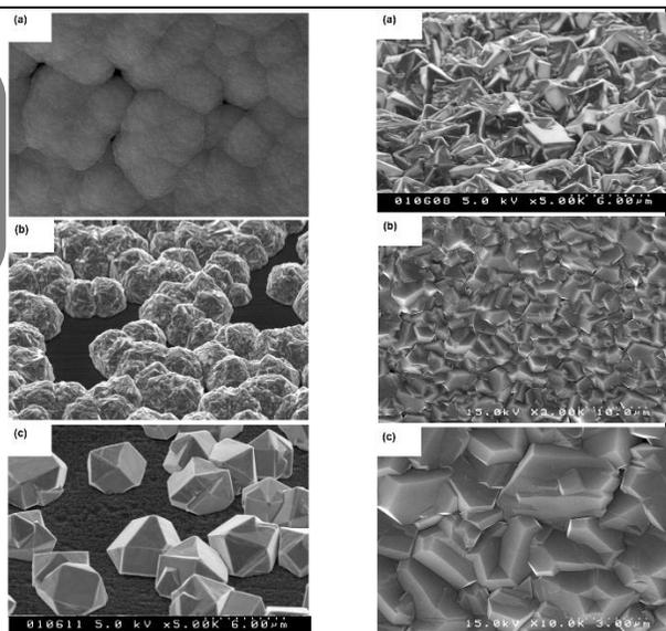
Fig. 2 SEM micrographs of the HFCVD diamond films grown at (a) 7sccm of (b) 5sccm and (c) 2 sccm of CH<sub>4</sub> in H<sub>2</sub> of about 93-98 sccm of H<sub>2</sub>. Right side images show micrographs of the HFCVD diamond films grown at substrate rotation of 10 rpm for (a) 6 hrs and 25 hrs respectively. Fig 2(c) is the magnified image of 2 (b).
