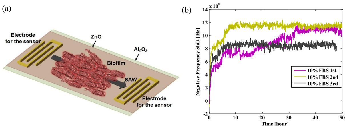
Fig. 3: (a) A schematic of the SAW sensor, (b) Resonant frequency shift results in three consecutive *E. coli* biofilm growth experiments in an animal serum (10% Fetal Bovine Serum) [4].
