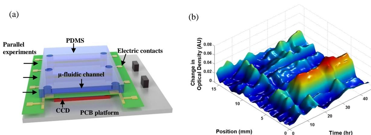
Fig. 2: (a) A schematic of the microfluidic platform with CCD components for spatiotemporal optical density measurements, (b) Surface reconstruction of biofilm morphology changes in the channel over time. Waterfall images are reconstructed using MATLAB based on the OD from the CCDs. The result illustrates the capability to investigate localized biofilm morphology differences [3].
