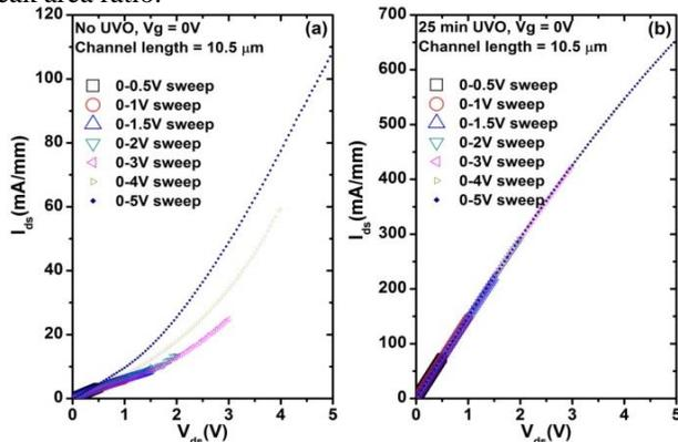
Fig. 5 Electrical stability measurement.
