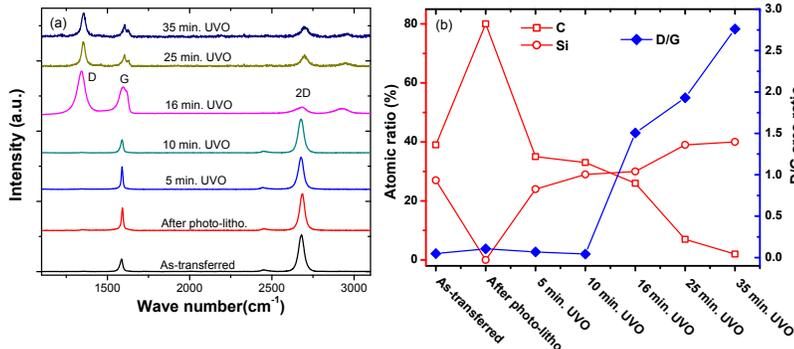
Fig. 2 Raman (a) and XPS characterization of the UVO treatment process. (b) left axis: atomic change, right axis: raman D peak to G peak area ratio.
