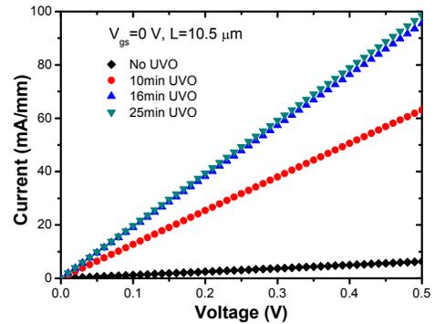
Fig. 3 I-V curve of devices with different UVO treatment time of the contact interface.
