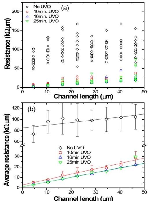
Fig. 4 (a) The statistical total resistance of devices underwent different UVO cleaning process. (b) Average total resistance corresponding to those in (a) and the TLM fitting.
