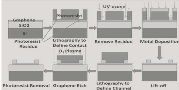
Fig. 1 Device fabrication process.
