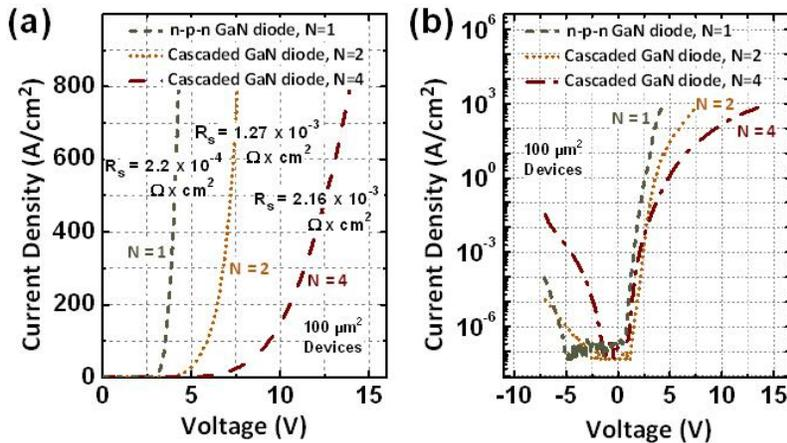
Figure 3. The experimental I-V characteristic of the cascaded p-n junctions with N=1, 3 and 4 (a) in linear scale (b) semi-log scale.
