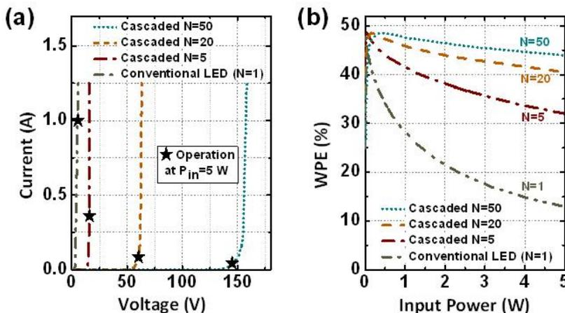
(a) I-V characteristic and (b) the change in wall plug efficiency as a function of input power of the modeled reference single junction LED and cascaded LEDs with N=5, 20 and 50.
