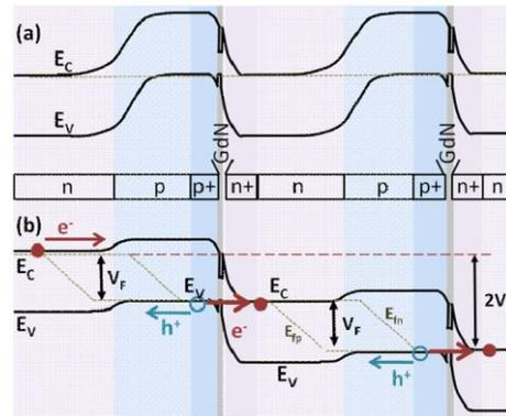
Figure 2. Energy band diagram of a cascaded p-n junction under (a) equilibrium (b) forward bias
