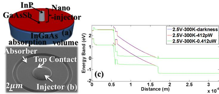
Fig. 1. **a** Device Schematic and **b**. SEM micrograph of a 10 $\mu$ m diameter injector showing the top metal contact, injector and absorber **c**. Energy band diagram along a vertical cutline through the central axis of device in darkness and under illumination.
