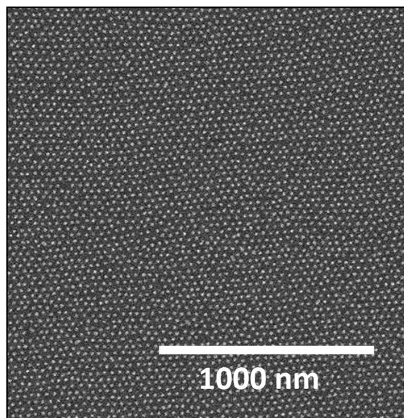
nanospheres arrayed over a block-copolymer templating film.
