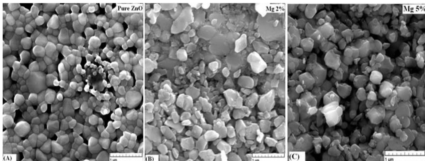
Figure 3: Scanning Electron Microscopy micrographs of  $\text{Mg}_x\text{Zn}_{1-x}\text{O}$  ( $x = 0, 2$  and  $5\%$ ) Systems
