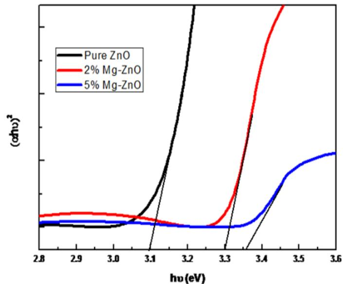
Fig 2: Calculation of band gap of  $\text{Mg}_x\text{Zn}_{1-x}\text{O}$  ( $x = 0, 2, 5\%$ ) by Tauc's Plot method.
