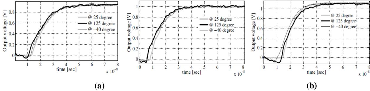
(c) **Fig. 8** The output response of the proposed comparator for a differential input signal of 50 mV for a VDD of (a) 0.9 V, (b) 1.0 V and (c) 1.1 V (under the temperature of -40 °C, 25 °C and 125 °C).
