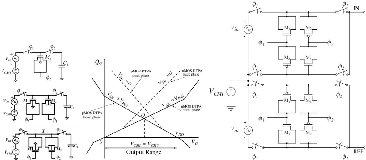
Fig.1 The schematic diagrams of the proposed preamplifier stage for the dynamic clocked comparator. Fig. 2 The Q-V characteristics of the anti-parallel connected parametric amplifier. Fig.3 The schematic diagram of the proposed preamplifier stage for the dynamic clocked comparator.
