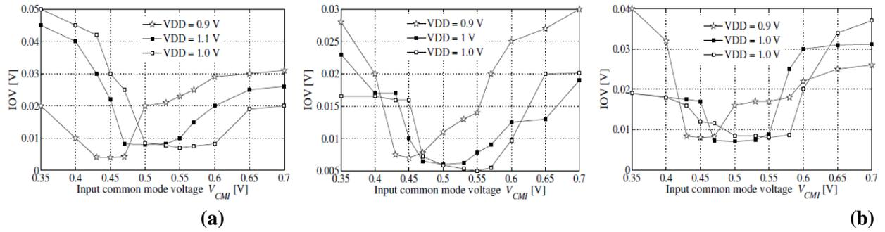
(c) **Fig. 7** The variation of an IOV with respect to  $V_{CM}$  at (a) 125 °C (b) 25 °C and (c) -40 °C (considering  $\pm$  10% variation in VDD).
