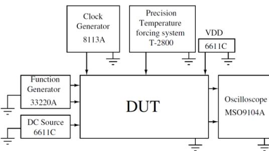
Fig.5 Microchip photograph. Fig.6 Test setup.
