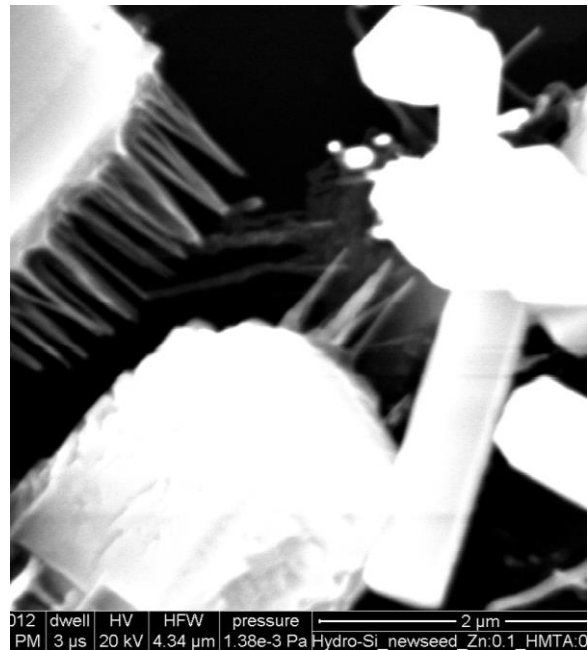
Figure 4 – SEM of ZnO nanowires core-shell structure seeded on top of ZnO NRs synthesized using hydrothermal method.
