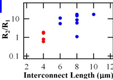
Figure 5 Changes in MLG resistivity by patterning to a width of 20 nm. Ratios of resistivity after patterning ( $R_2$ ) to the original one ( $R_1$ ) as a function of the interconnect length are shown. The resistances of interconnects with a length of 4 μm did not change by patterning, while those of interconnects longer than 6 μm tended to increase after patterning.
