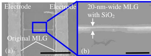
Figure 4 (a) SEM image of 20-nm-wide intercalated MLG interconnect with a length of 6 μm. The scale bar is 2 μm. (b) Enlarged SEM image of the interconnect. Isolated 20-nm-wide graphene with 70-nm-thick SiO<sub>2</sub> (HSQ) used for EB mask is clearly observed. The scale bar is 200 nm.
