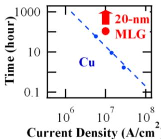
Figure 6 Time to failure for the 20-nm-wide intercalated MLG with a length of 4 μm and a thickness of ~3.7 nm (11 graphene layers) is shown as a red colored circle. The MLG at a current of  $1 \times 10^7$  A/cm<sup>2</sup> at 250°C did not break over 110 hours, showing that the graphene interconnect has higher reliability than Cu with a width of 160 nm, as shown in blue [3].
