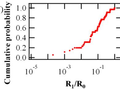
Figure 3 The cumulative probability distribution of the ratios of the sheet resistance of intercalated MLG for 38 hours ( $R_1$ ) to the original ( $R_0$ ).
