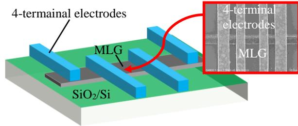
Figure 2 Schematic diagram of a MLG interconnect. The MLG was evaluated with four-terminal electrodes which were composed of Ti/Au. A SEM image of the MLG interconnect is shown in the inset.
