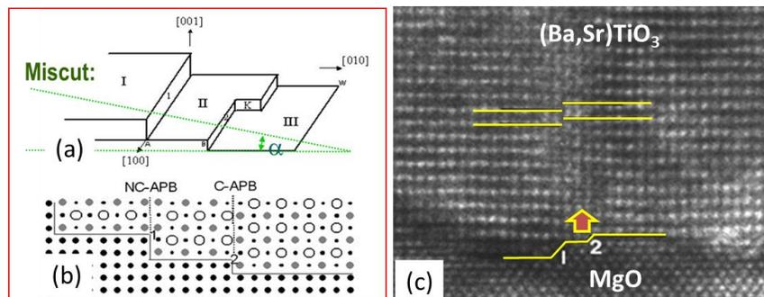
Figure 1 Illustration of the substrate surface (a) showing steps, terraces and kinks and (b)  $(\text{Ba,Sr})\text{TiO}_3/\text{MgO}$  interface along the  $[100]_{\text{MgO}}$ . (c) HRTEM image of  $(\text{Ba,Sr})\text{TiO}_3/\text{MgO}$  interface.
