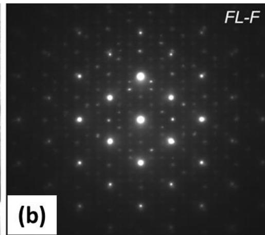
Figure 4 (a) Cross-section TEM and (b) electron diffraction pattern of a  $\text{Mn}:(\text{Ba},\text{Sr})\text{TiO}_3//\text{Mn}:\text{Ba}(\text{Zr},\text{Ti})\text{O}_3$  multilayered structure.
