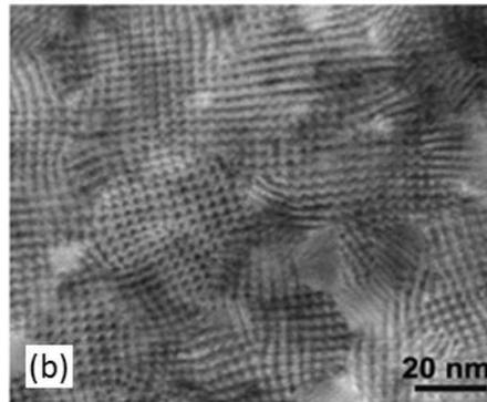
Figure 3 (a) Electron diffraction pattern and (b) HRTEM image of a 2-D  $(\text{Ba},\text{Sr})\text{TiO}_3/\text{MgO}$  interface.
