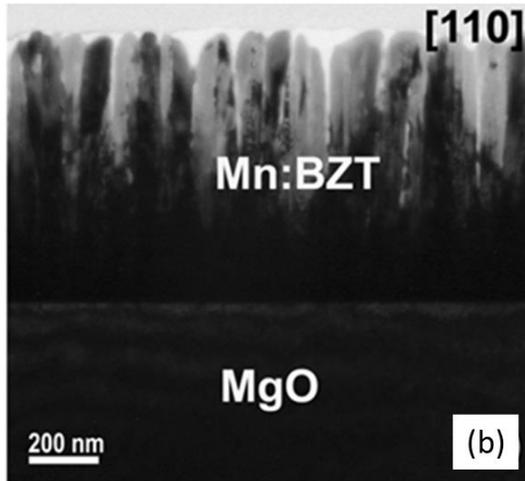
Figure 2 (a) Illustration of four types of twins formed by joining  $\{111\}$ . (b) XTEM of  $\text{Ba}(\text{Zr},\text{Ti})\text{TiO}_3/\text{MgO}$  showing nanofinger structures.
