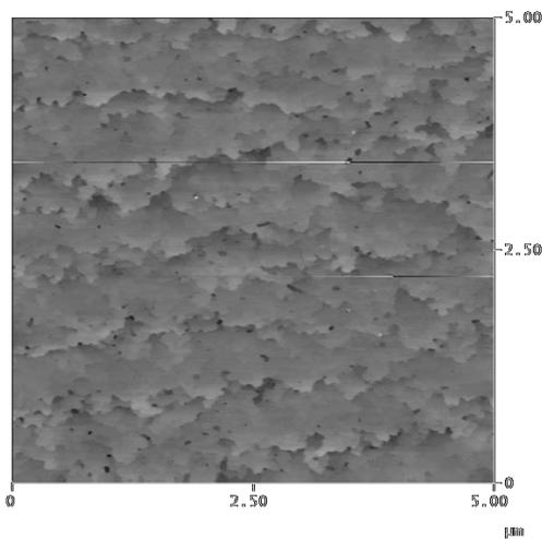
Figure 2. Atomic force microscopy image of AlN on sapphire. RMS surface roughness is 1.021 nm. Z-scale is 20 nm.
