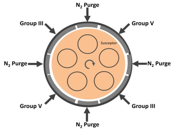
Figure 1. Schematic of MOCVD chamber showing spatially separated group III and group V injection ports.
