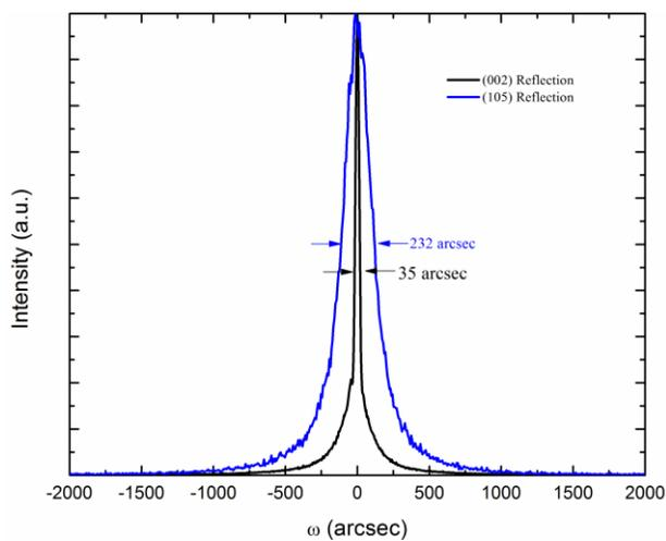
Figure 3. High resolution x-ray diffraction rocking curves of the (002) and (105) reflection.
