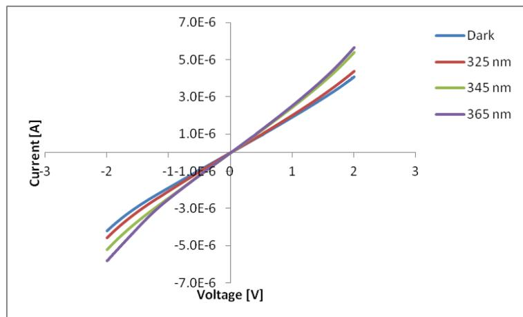
Figure 2. The IV characteristics of a ZnO/p-Si Schottky diode grown at high oxygen overpressure and 300 °C. The differences between dark and light ( $\lambda=320, 345,$  and  $365$  nm) responses of this device are evident.
