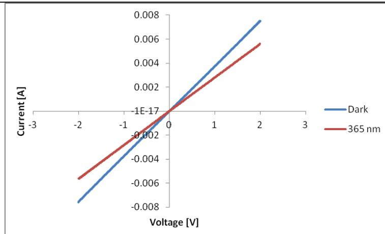
Figure 1. The IV characteristics of a ZnO/n-Si photoresistor grown at low oxygen overpressure and 300 °C. The response of the device is derived at 365 nm.
