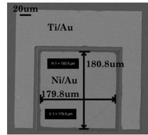
(b) SEM top view of finished InN device
