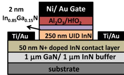
(a) Cross-section schematic of InN MOSCAP
