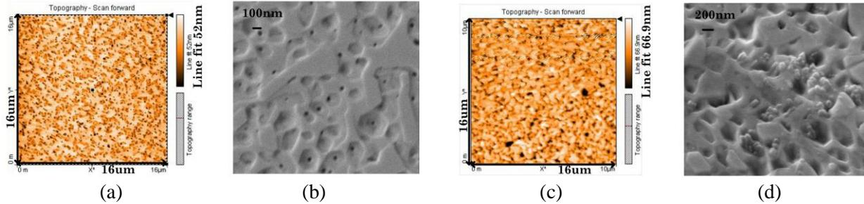
Fig.2 AFM (a) and SEM (b) of InN surface; AFM (c) and SEM (d) of oxide surface on InN
