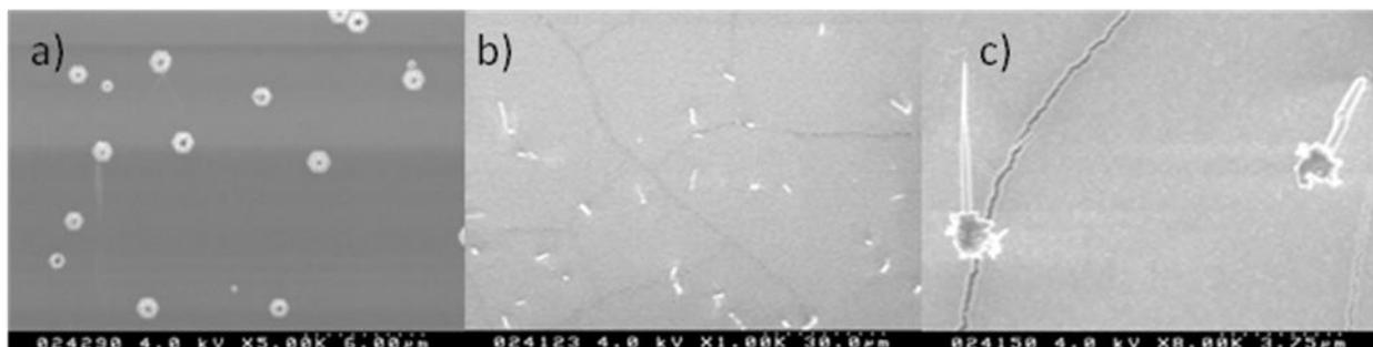
Figure 2: AFM topographs of GaN surface a) before anneal, b) after 1150 °C anneal for 30 minutes and c) after 1300 °C anneal for 30 minutes with the AlN capped removed by 2M KOH solution.
