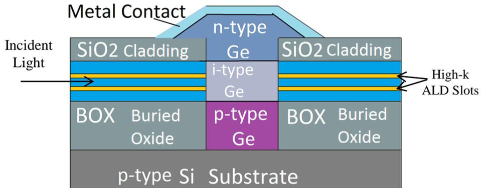
Fig.1. Schematics of the waveguide-detector junction. The detector mesa is grown after fabrication of the waveguides. A PIN diode is formed using epitaxy. The incident light will face the intrinsic germanium to maximize the quantum efficiency.
