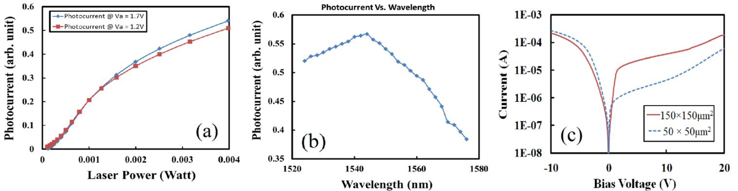
Fig.4. Shows the photocurrent measurements versus (a) laser power at 1.2V and 1.7V bias, and (b) laser wavelength at 1.2V bias. (c) Shows the current measurements in darkness.
