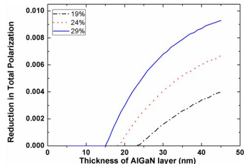
Figure 4 Reduction in effective total polarization in AlGaIn layer versus thickness for different Al contents. Beyond the critical thickness, the piezoelectric polarization weakens owing to strain relaxation and the total polarization tends towards the spontaneous polarization value.
