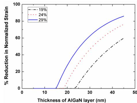
Figure 3 Calculated % reduction in normalized strain present in AlGaIn layer for three different Al compositions. At large Al content, strain relaxation occurs at lower thickness and dislocations form to reduce strain energy
