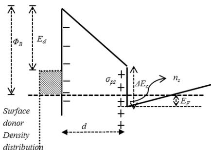
Figure 2 Band diagram of typical structure of a AlGaIn/GaN HEMT.  $\Phi_b$  is the surface barrier height (SBH).
