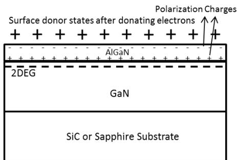
Figure 1 Typical structure of a AlGaIn/GaN HEMT showing various charges at the different interfaces and illustrating the formation of 2DEG with electrons supplied by surface donor states.
