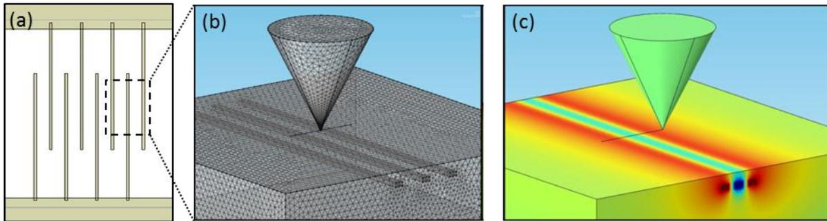
Fig.1 (a) Test structure layout (Part), (b) Meshing of Simulation Geometry, (c) Visualization of the Electric Potential.
