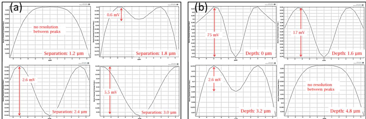
Fig.2 (a) Surface Potential Distribution at Various Wire Separations, Wires at 4.8  $\mu\text{m}$  Depth,
