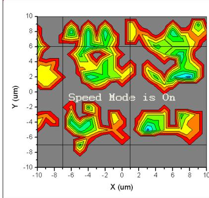
Fig 3 SEU Mapping of the DICE SRAM
