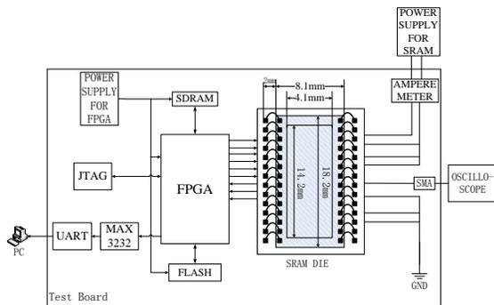
Fig 1 Laser test Print Circuit Board (PCB)
