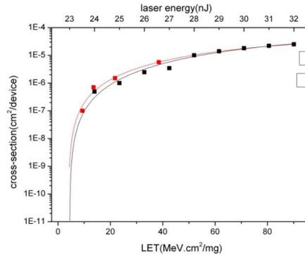
Fig 4 The Cross Section of Heavy ion (the curve with red color) and pulsed laser (the curve with black color)
