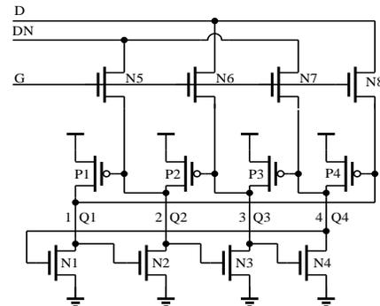
Fig 2 Schematic of the DICE cell
