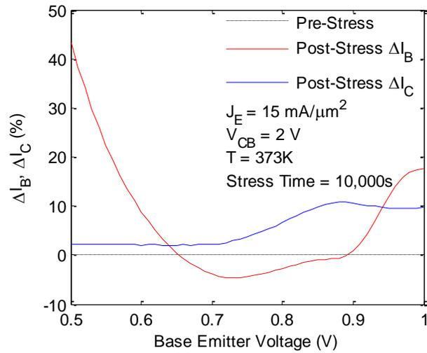
Fig. 1. Change in base current from the SiGe HBT Gummel characteristics after high current stress.
