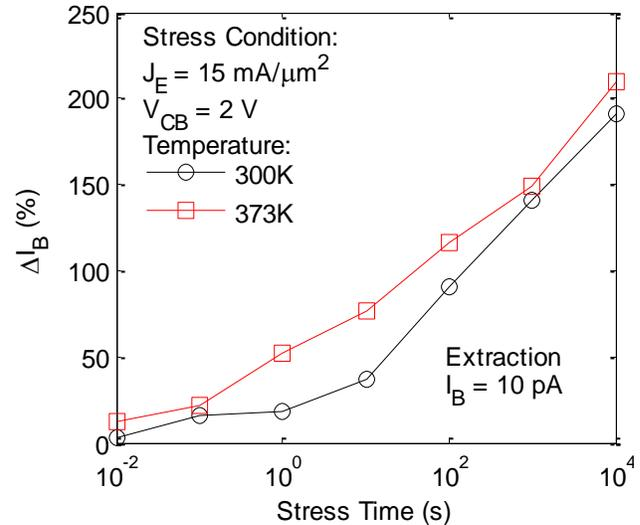
Fig. 4. Base current evolution at  $I_B = 10\text{ pA}$  for different temperatures under high current stress.
