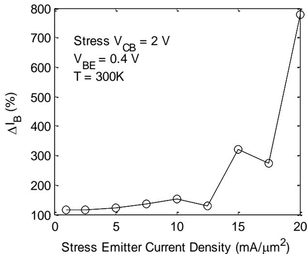
Fig. 3. Threshold behavior of base current degradation around  $10\text{mA}/\mu\text{m}^2$ .
