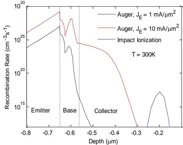
Fig. 2. Auger generation and impact ionization rate cross section at high current densities from TCAD.
