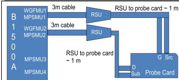
Figure 1: Schematic of the measurement setup (not to scale)
