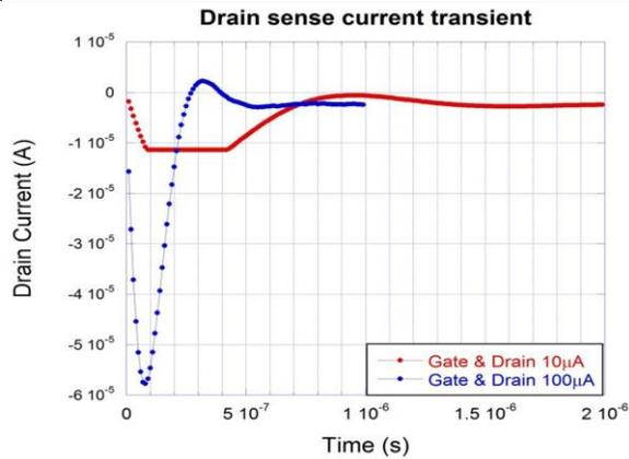
Figure 5: Impact of current compliance limit on settling time of the MOSFET.
