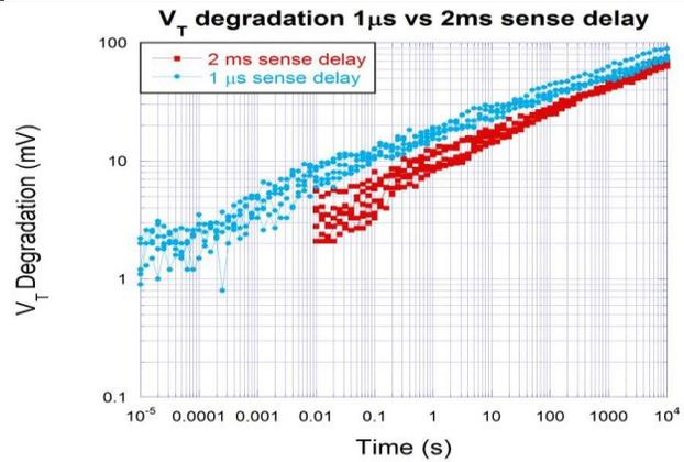
Figure 6: Impact of sense delay on  $V_T$  degradation.
