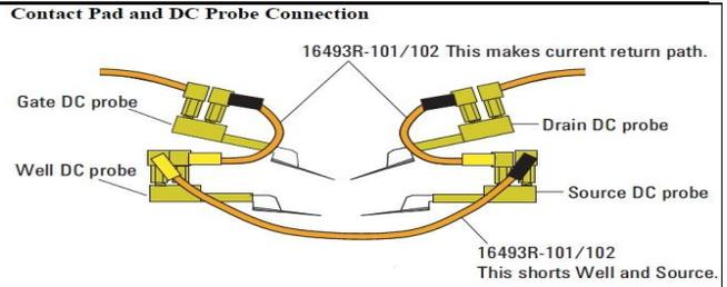
Figure 2: Measurement setup suggested by Agilent for fast measurements. [4]
