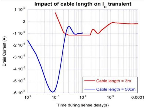
Figure 3: Impact of reducing the cable length from the RSU to the probe card.
