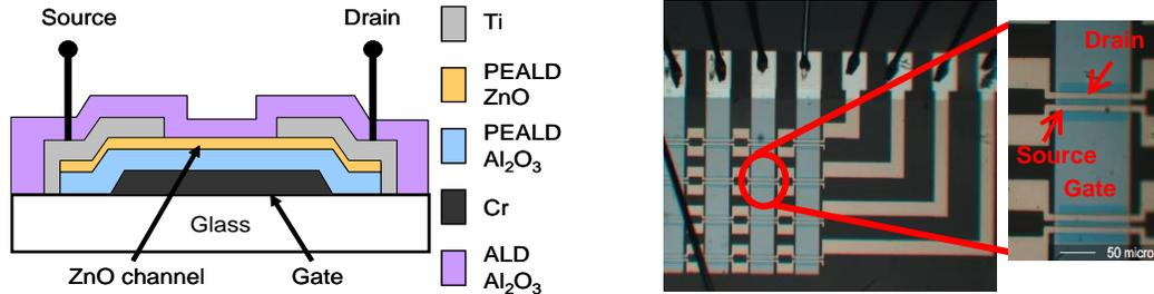
Fig. 1: (left) Bottom gate ZnO TFT schematic cross section; (right) optical micrograph of 4 x 4 ZnO TFT array used in electrical bias and radiation measurements
