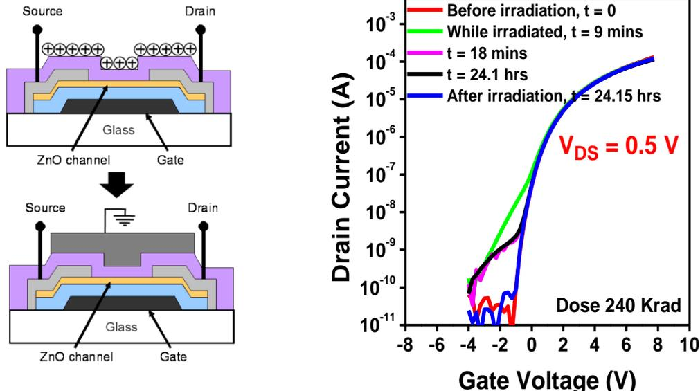
Figure 3: (left) Bottom-gate TFT structure collects ionized charge on the channel back interface. Back channel was grounded to avoid ionized charge to be collected. (right) Linear region ( $V_{ds} = 0.5$  V)  $\log(I_D)$  versus  $V_{GS}$  for a cumulative  $^{60}\text{Co}$  dose of 240 Krad with the back channel surface grounded to avoid collection of charge at the surface.
