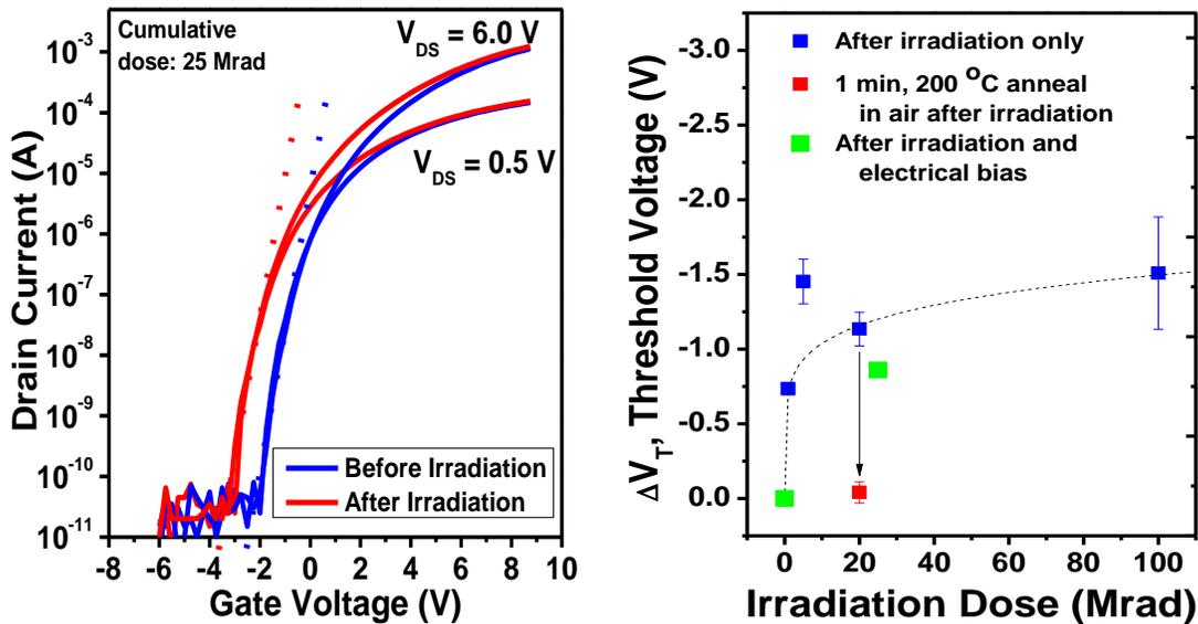
Fig. 2: (left) Linear region ( $V_{ds} = 0.5$  V) and saturation region ( $V_{ds} = 6$  V)  $\log(I_D)$  versus  $V_{GS}$  of ZnO TFTs pre- and post- irradiation for a cumulative  $^{60}\text{Co}$  dose of 25 Mrad. Device dimensions are  $W/L = 100 \mu\text{m}/5 \mu\text{m}$ . (right) Threshold voltage as a function of irradiation dose for irradiation only and irradiation with electrical bias. In both cases, threshold voltage shift is similar.
