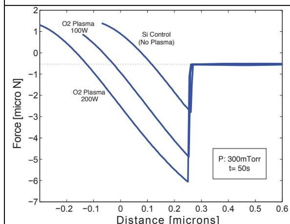
**Fig. 3** Force spectroscopy of unexposed and plasma activated Si surfaces obtained using SiO<sub>2</sub> sphere contacts.
