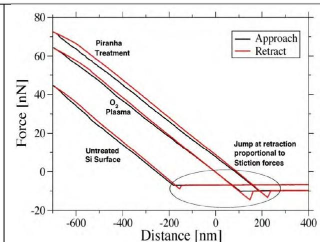
**Fig. 2** Force-Distance curves measured using AFM on surface (plasma & piranha) activated and untreated samples.
