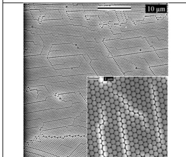
**Fig. 5** SEM image showing monolayer of PS spheres in Fig.4 produced on plasma activated Si via drop coating.
