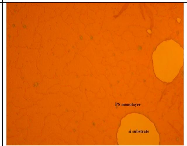
**Fig. 6** Optical Image (×200) showing a monolayer of spin-coated PS spheres ( $d=0.5\mu\text{m}$ , 4%w/v) diluted
