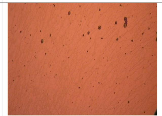
**Fig. 4** Optical image (×200) showing a monolayer of drop-coated PS spheres ( $d=0.5\mu\text{m}$ , 2.5%w/v) diluted 1:1 in ethanol.
