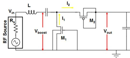
Figure 1. Voltage doubler using diode-connected MOSFETs.
