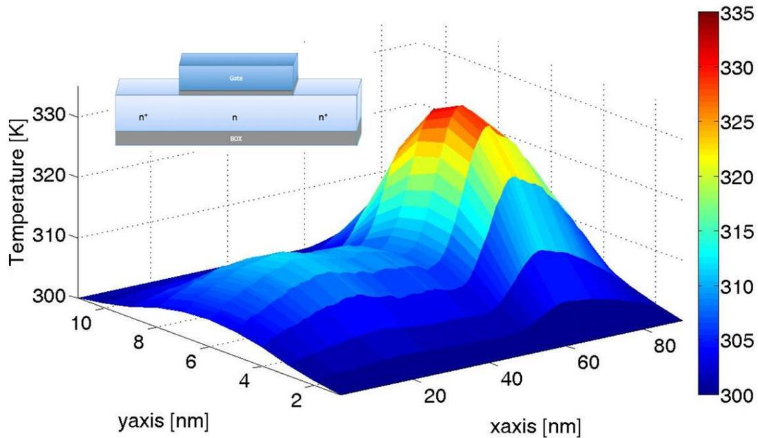
Figure 2: Temperature profile of a junctionless transistor with a 5nm square cross-sectional length and  $L_G = 20 \text{ nm}$ . Inset: Schematic of a junctionless transistor.
