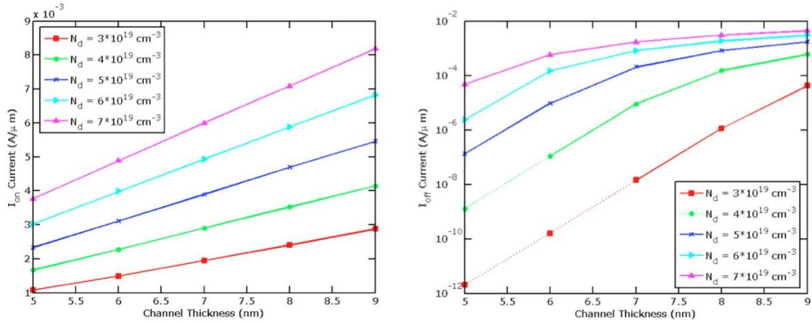
Figure 1:  $I_{on}$  (left) and  $I_{off}$  (right) current of junctionless transistors as a function of channel thickness and doping concentration.  $L_G = 20 \text{ nm}$ ;  $V_G = V_D = 1.2 \text{ V}$ .
