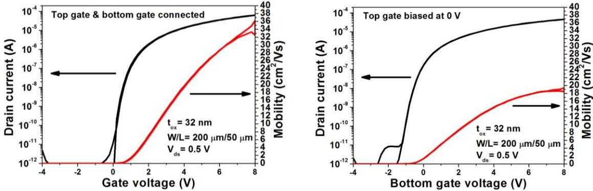
Fig. 2 Linear region drain current (log scale) and field-effect mobility (linear scale) versus gate voltage of PEALD double-gate tri-layer TFT with (left) top and bottom gates connected together and (right) bottom gate swept with top gate held at 0 V.
