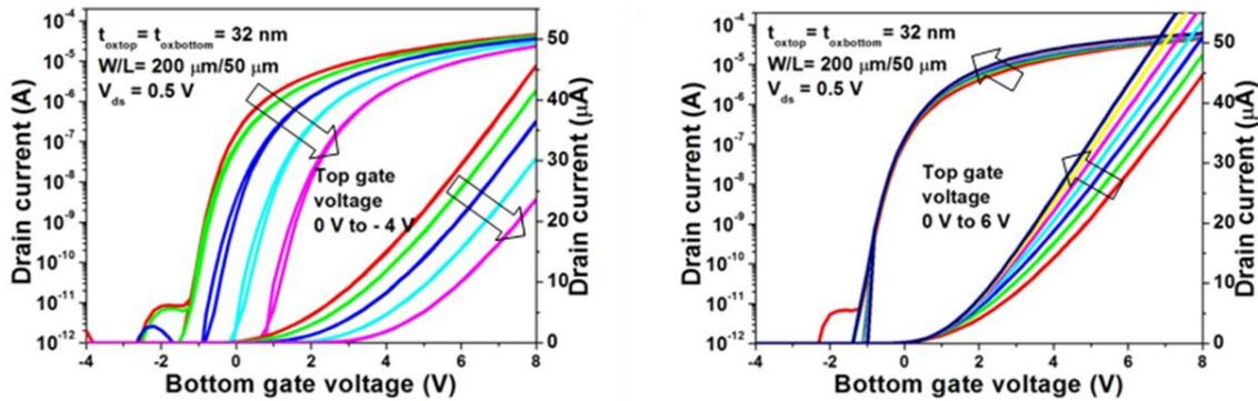
Fig. 3 Drain current versus bottom gate voltage of PEALD double-gate tri-layer TFT with top gate voltages of (left) 0 V to -4 V and (right) 0 V to 6 V.
