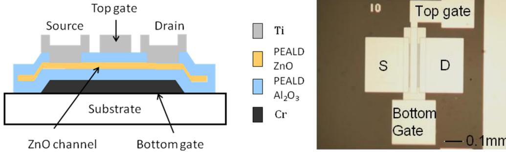
Fig. 1 (left) PEALD double-gate tri-layer TFT cross-section, (right) microscope image of PEALD double-gate tri-layer TFT.
