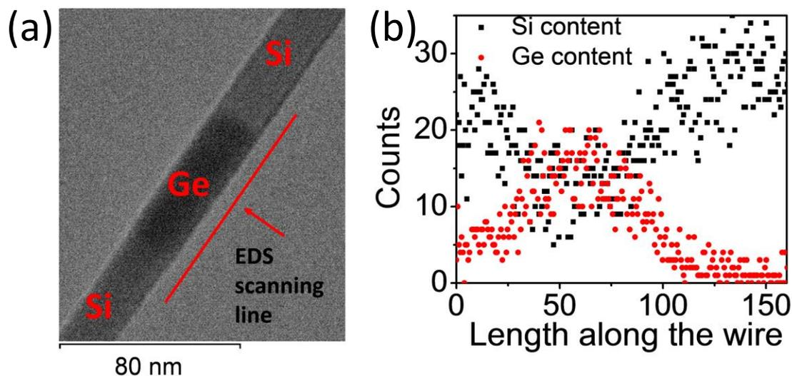
**Figure 3:** (a) TEM image of the Si/Ge/Si hetero-NW p-n junction of  $D \sim 20$  nm, grown at Los Alamos National Lab. (b) EDS analysis of the hetero-NW confirms the composition modulation along the wire, from Si to Ge to Si.
