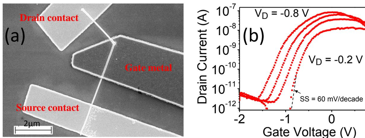
**Figure 2:** (a) SEM image of the SiGe hetero-NW TFET with  $D \sim 50$  nm, grown at Los Alamos National Lab. (b)  $I - V$  characteristic of the device in tunneling operation mode at  $T = 300$  K.
