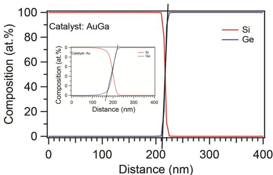
**Figure 1:** Composition profiles, obtained from atom probe tomography (APT) analysis, of the SiGe heteronanowire grown from AuGa alloy catalyst ( $\sim 9$  nm heterojunction width); inset: the SiGe heterojunction grown from Au catalyst for comparison ( $\sim 44$  nm heterojunction width).
