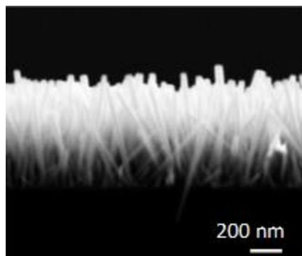
Figure 1a. Uncoated ZnO nanowires
