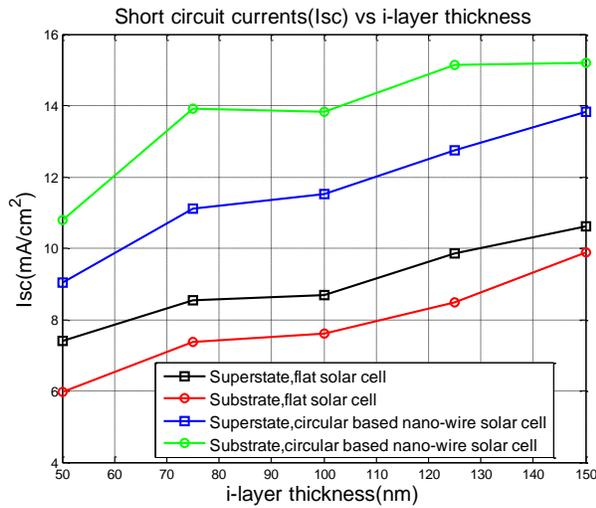
Figure 2. Jsc of different pin diode structures
