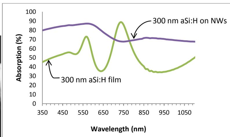
Figure 1b. Reflectance spectra of 300 nm aSi:H coated on nanowires and 300 nm aSi:H planar film
