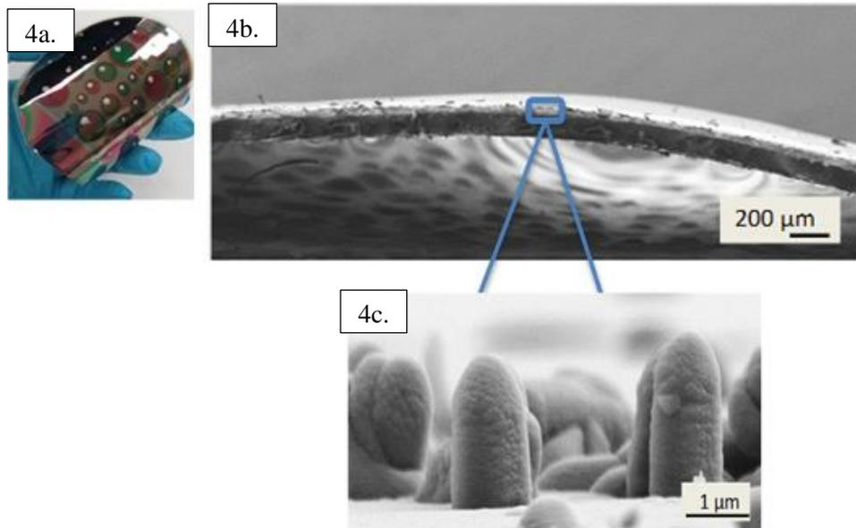
Figure 2a. Optical image of hybrid ZnO nanowire/aSi:H thin-film solar cells on a flexible substrate; b. SEM image of the flexed substrate with hybrid nanowire devices, and c. SEM micrograph of the hybrid nanowire devices.
