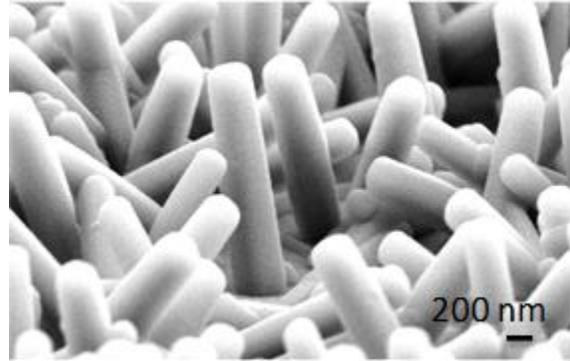
Figure 3. 300 nm aSi:H shell/ZnO core nanowires
