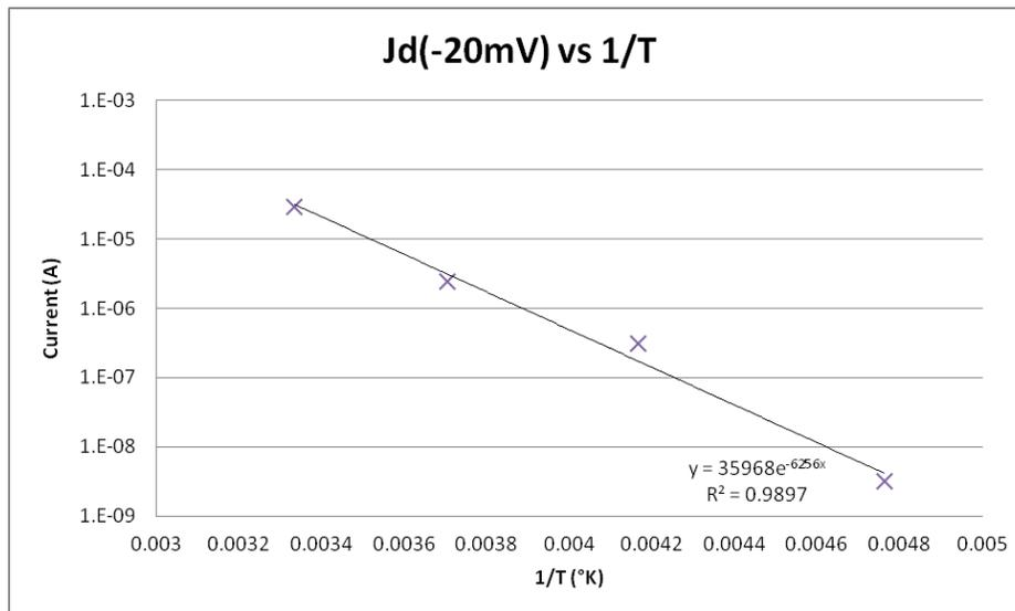
Figure 2. Dark current measurement vs 1/T for 250  $\mu\text{m}$  diodes
