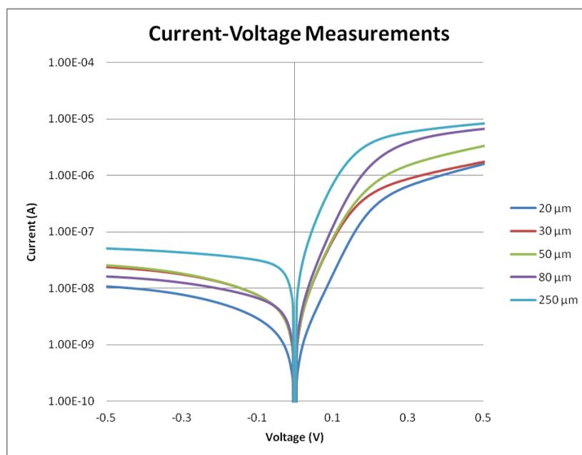
Figure 1. I-V measurements of various diameter diode at 300°K
