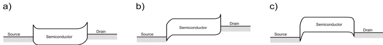
**Figure 1: Three possible operational states. a) Thermionic Emission (TE) at both junctions, b) TE and tunneling (TU) at the source and TE at the drain junction, c) an additional tunneling barrier at the drain junction.**
