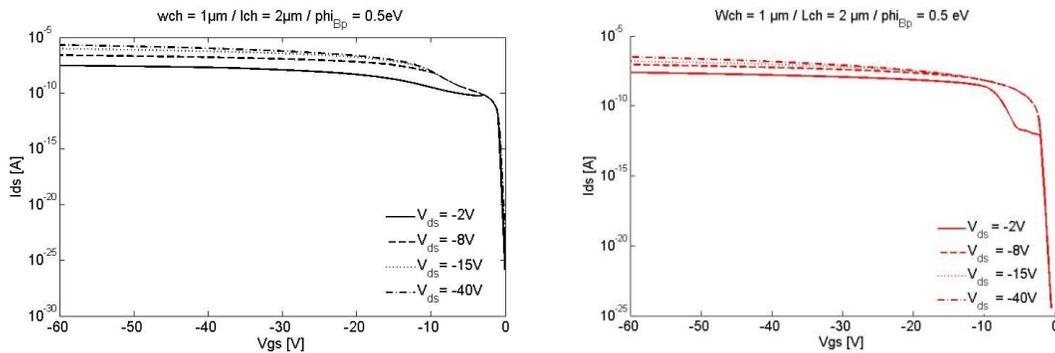
**Figure 2: Simulated (TCAD sentaurus) (left) and modeled (right) transfer characteristic with a barrier height of 0.5eV. The kinks can be clearly related to the transport mechanisms at the source and drain junctions.**
