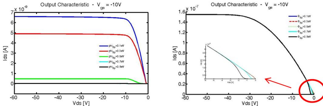
**Figure 4: Simulated (left) and modeled (right) output characteristic for various barrier heights.**
