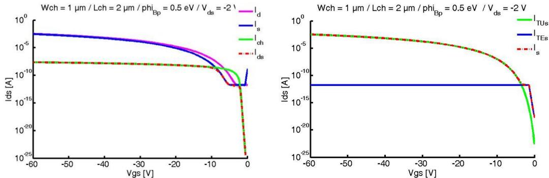
**Figure 3: Total current limitation by either the source drain injection current or the channel current (left). The source current consists of a TE and a TU part. At higher barriers the source contribution develops a kink.**
