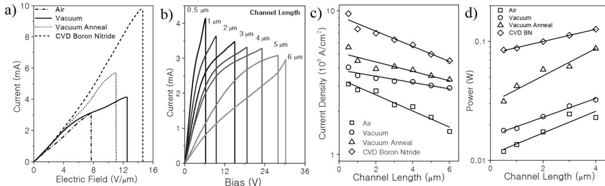
Figure 3: (a) Comparison of device breakdown at high-fields for 500 nm channel length devices. b) Breakdown characteristics of graphene ribbons of varying channel length. (c) Maximum current density of devices before breakdown. (d) Sustained power before device breakdown.
