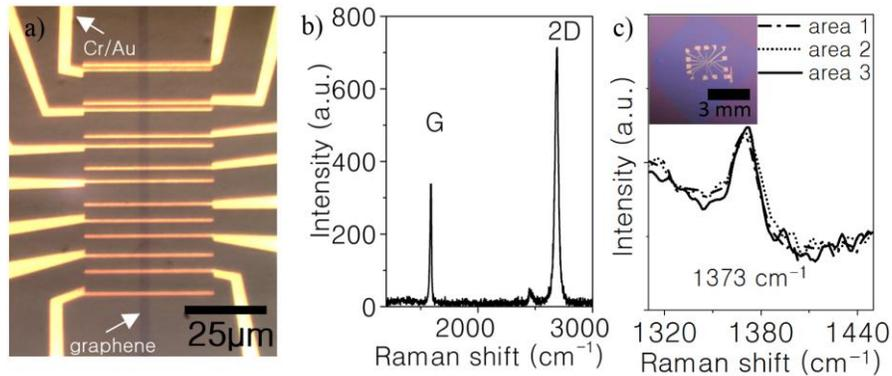
Figure 1. a) Optical micrograph of a 3  $\mu\text{m}$  wide graphene ribbon contacted in the TLM configuration on 285 nm SiO<sub>2</sub>. b) Raman spectra of post-fabricated device. c) Raman spectra of CVD hBN (three different areas) showing the characteristic peak centered near 1373  $\text{cm}^{-1}$ . (inset) Large-area CVD hBN stack (5 layers) used as the substrate (appears dark purple) with TLM design patterned using ebeam lithography.
