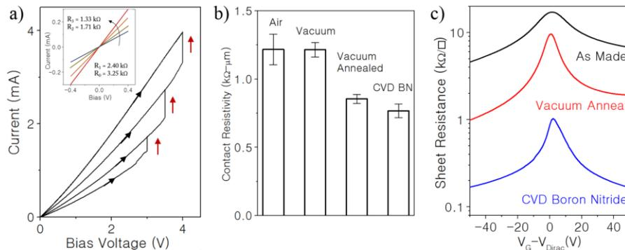
Figure 2: a) Current-voltage trace of consecutive high vacuum current annealing runs on the same graphene device. Bias is held at 3.0 V, 3.5 V, and 4.0 V for 10 min. b) Contact resistivity extracted from TLM measurements showing a  $\sim 30\%$  decrease after current annealing. c) Sheet resistance as a function of gate voltage for graphene devices before/after high vacuum current annealing and post-annealed on a pentalayer CVD hBN substrate.
