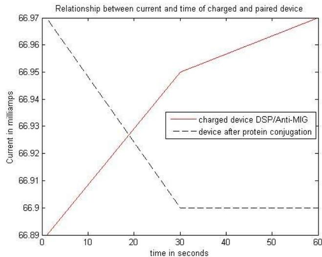
**Fig. 3:** Behavior of Drain Current  $I_D$  before and after protein conjugation. The changes in current can be compared to clean device steady state current of 66.89mA.
