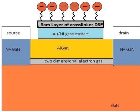
**Fig. 1:** Visualization of the device when it is ready to use. The addition of Anti-MIG antibody induces additional negative charges to the channel which results in an increase in drain current.
