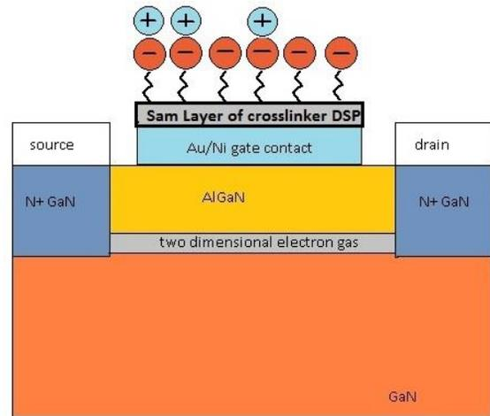
**Fig. 2:** Visualization of the device once conjugation between protein and antibody has taken place. The positive charges of the MIG introduced to the channel pair with electrons gained in the previous step.
