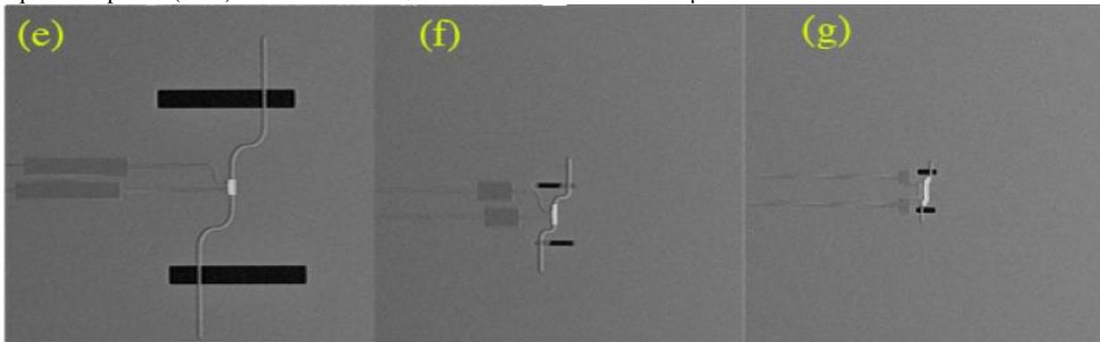
(e), (f) and (g) are images of 300 GHz, 1 THz, and 3 THz devices, respectively. A thin layer of Bi is deposited to act as an radiation absorber.
